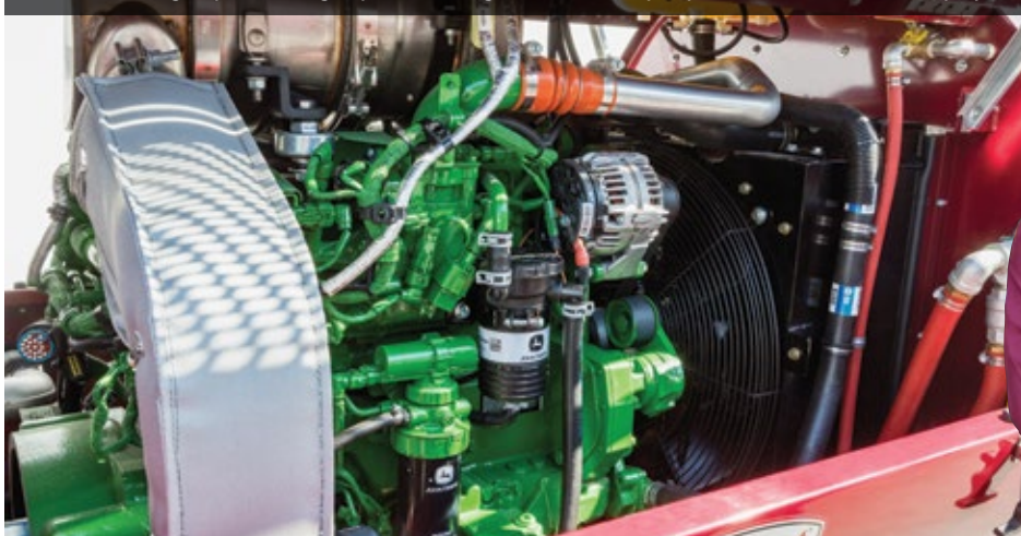
A John Deere engine powers a high-speed centrifugal fan and water pump on the LectroBlast 2650 sprayer.
